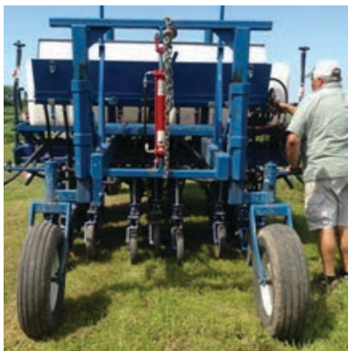
Penn State cover crop inter-seeder and applicator.
