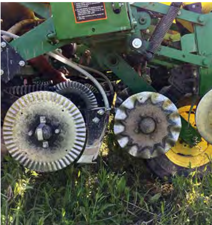
Figure 15. The fertilizer dispenser behind the ripple coulter on this planter (left) caught cereal rye residue while no-till planting soybean (right), which reduced mulch uniformity and interfered with seed placement.
