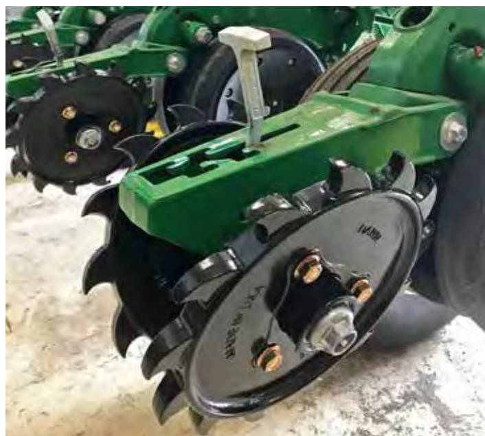
Figure 21. Gaguetine closing wheels crumble the soil while zipping the furrow shut.
