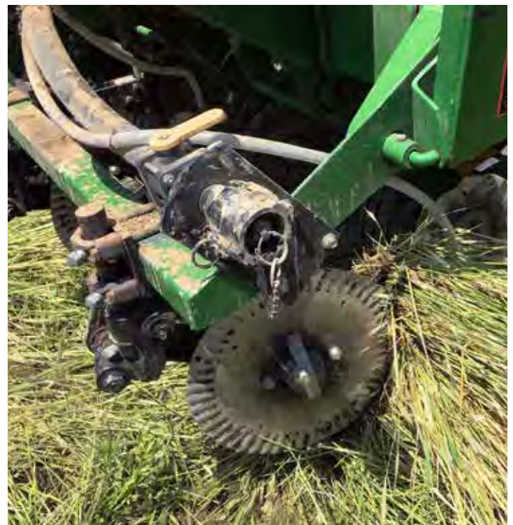
Figure 15. The fertilizer dispenser behind the ripple coulter on this planter (left) caught cereal rye residue while no-till planting soybean (right), which reduced mulch uniformity and interfered with seed placement.
